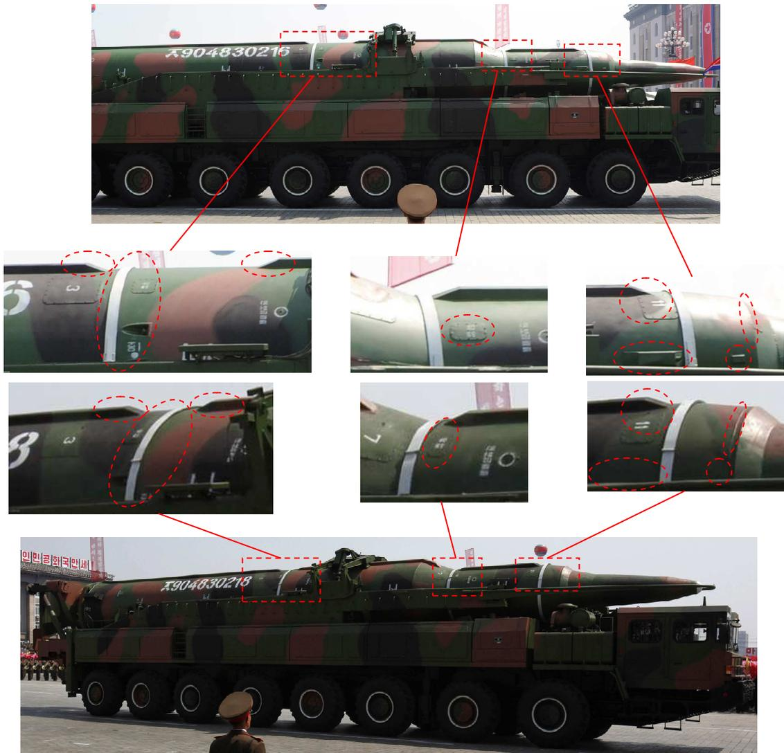
**Figure 3: Examples for Different Details on KN-08 Missiles**
